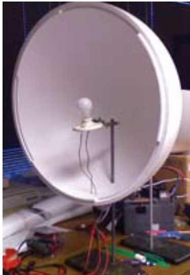
Garber's class student-made intergrating sphere.
