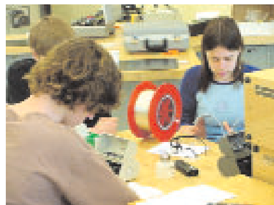
Photonics Technology students work with both single and multimode fiber, generously donated by OFS’s Sturbridge Optical Fiber Division. Here, they learn to create flat fiber end faces with YORK cleavers (white and grey units on either side of fiber spool). Reading the manual before beginning work speeds the process!
