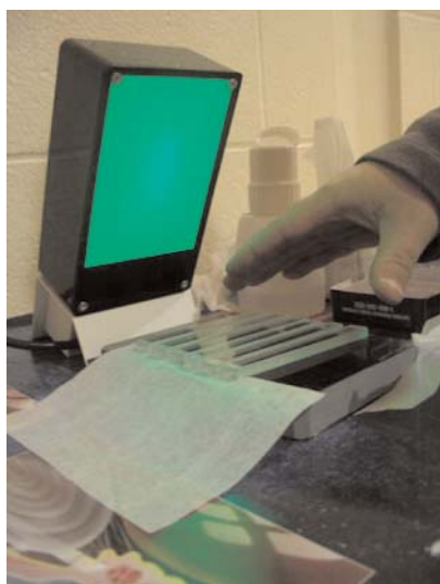
TRCC students use a green inspection lamp to look at interference fringes caused by an air film trapped between flat glass plates.
